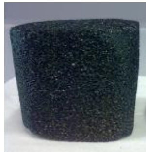
Polymeric foam cured at 150°C
