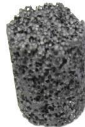
Carbon foam pyrolysed at 1000°C
